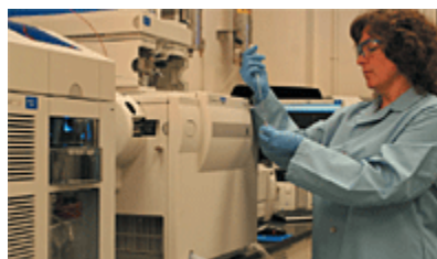
A Pacific Northwest National Laboratory (PNNL) scientist works on the capillary electrophoresis electrospray ionization ion trap mass spectrometer (CE/ESI/MS). This instrument is designed to efficiently separate and detect a range of analytes. (Source: PNNL)
