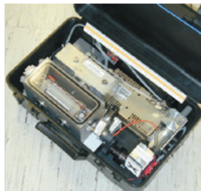
A suitcase-sized MALDI-TOF mass spec instrument can be used to detect bioterror agents. (Source: Andrew Feldman, PhD)
